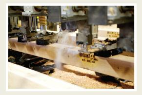
To ensure that every crossarm meets our high standards, we've incorporated this test into our manufacturing process. As it passes through our automated drilling process, each crossarm gets stamped with an electric load cell, pre-programmed to apply up to 1,900 pounds of stress.
