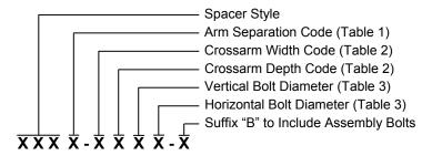
**Ordering Example:** 5861-3345-B = 586 Series Adjustable Spacer Fitting Style with  $10\frac{3}{4}$ " to  $14\frac{3}{4}$ " arm separation adjustment for  $3\frac{5}{8}$ " x  $7\frac{1}{2}$ " side arms. The spacer fitting is tapped for and furnished with (2)  $\frac{1}{2}$ " vertical and (4)  $\frac{5}{8}$ " horizontal assembly washer head bolts.
